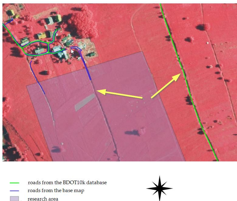
Figure 13. Elements of the road network in the area of Rycerka Górna against the background of the orthophotomap. Source: Own study.
