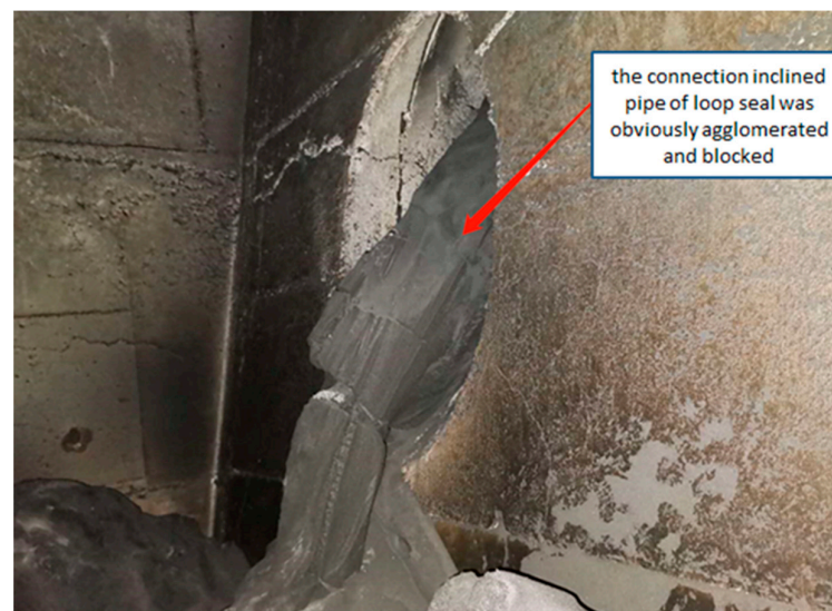
Figure 4. Loop seal blockage.
