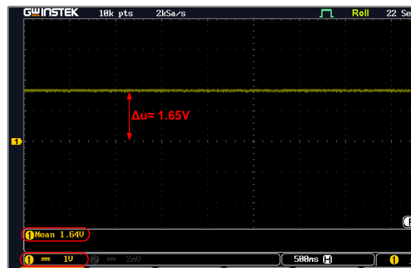
Figure 5. The output voltage of the INA241A2 amplifier in the absence of input voltage (amplifier supply voltage V_s = 3.3 V).
