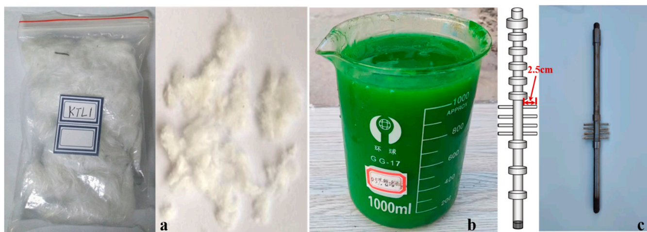
Figure 2. Diagram of fiber fracturing fluid and wellbore: (a) fiber used for configuring fiber fracturing fluid; (b) fiber fracturing fluid with tracer added; and (c) wellbore in perforated mode.
