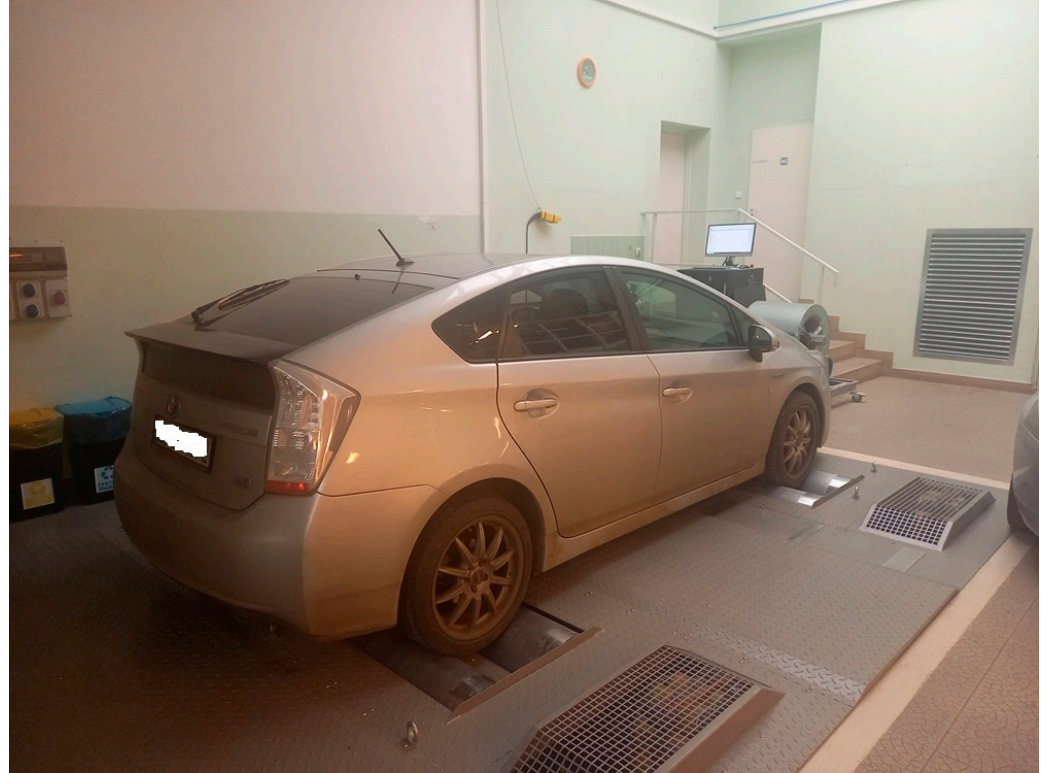
Figure 3. Tested vehicle on V-tech VT4/B2 chassis dynamometer.
