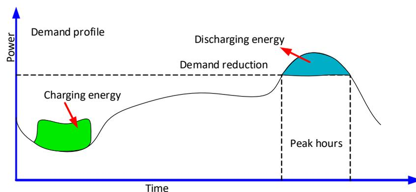
Figure 12. Load profile where the ESS is used to reduce the peak demand.
