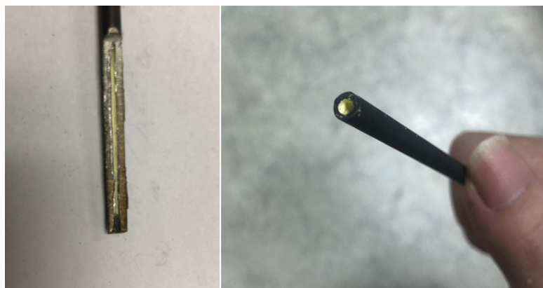
Figure 3. Section and cross-section of catalyst coating.
