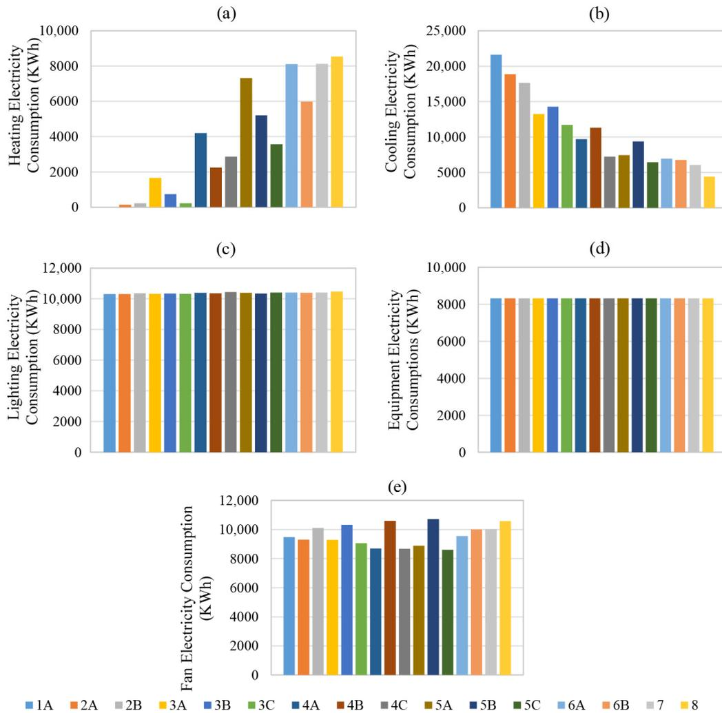
**Figure 7.** Average annual energy consumption of end-use systems for various climate zones. (a) Heating electricity consumption; (b) Cooling electricity consumption; (c) Lighting electricity consumption; (d) Equipment electricity consumption; (e) Fan electricity consumption.
