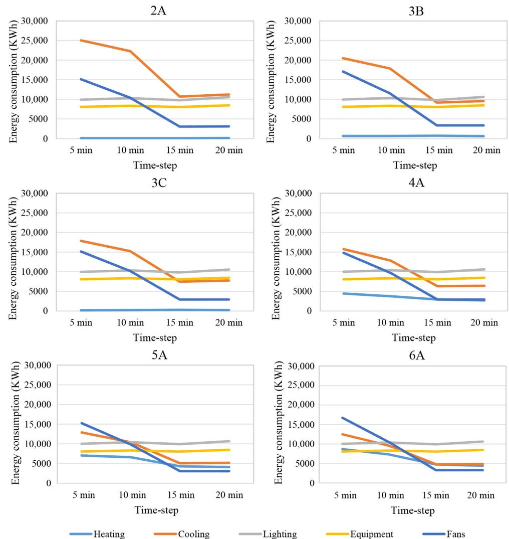
**Figure 11.** The impact of occupancy simulation time-step size on building energy performance.
