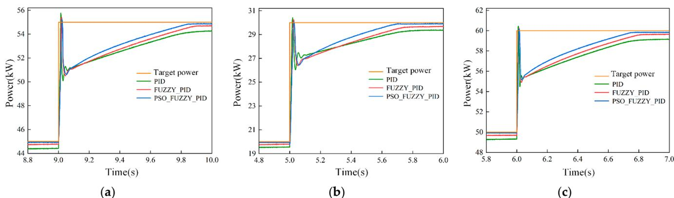
**Figure 15.** Target power tracking effect of three control strategies under different transitional conditions: (a) 45–55 kW in working condition 1; (b) 20–30 kW in working condition 2; (c) 50–60 kW in working condition 3.
