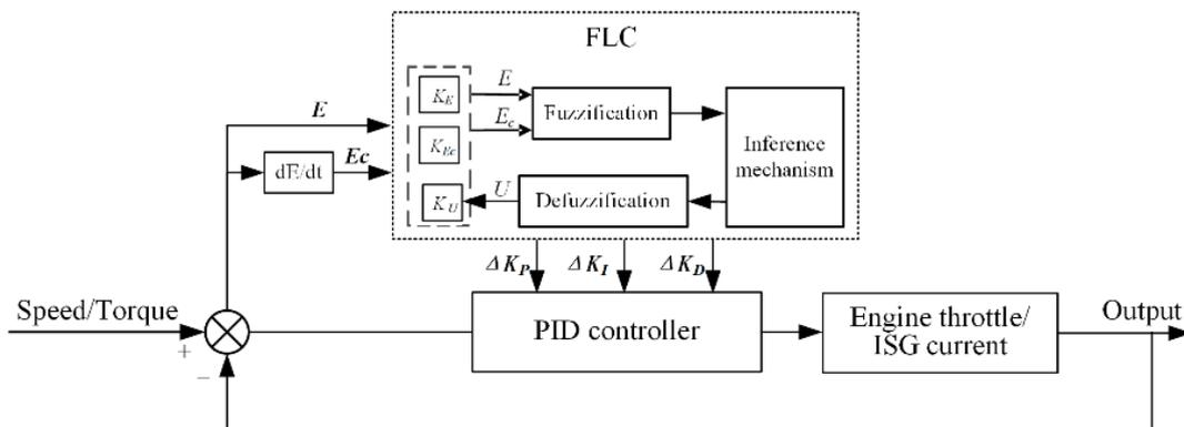
Figure 7. Schematic of fuzzy PID control algorithm.
