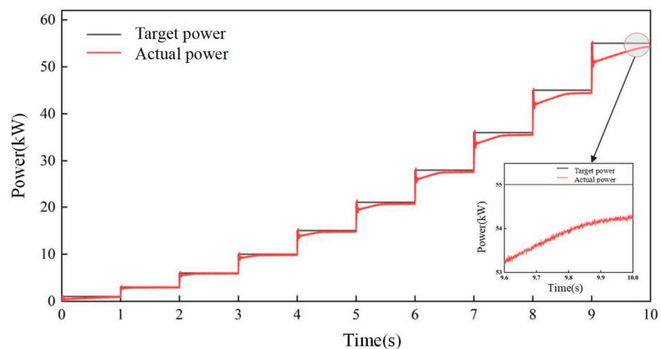
Figure 14. Power response of HIL test.
