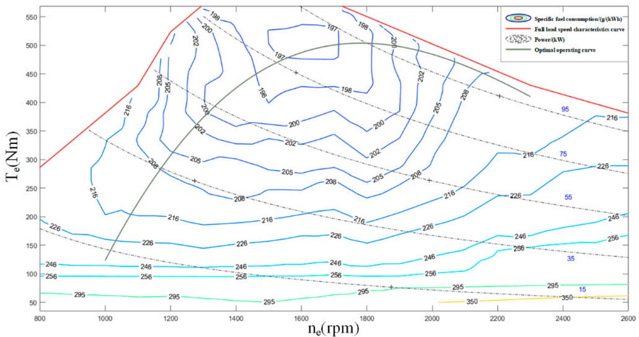
Figure 5. APU fuel consumption characteristics map and the optimal operating curve.
