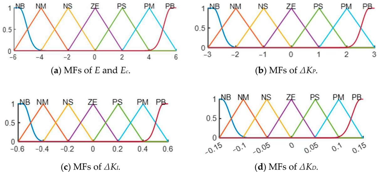
Figure 8. MFs of inputs and outputs.
