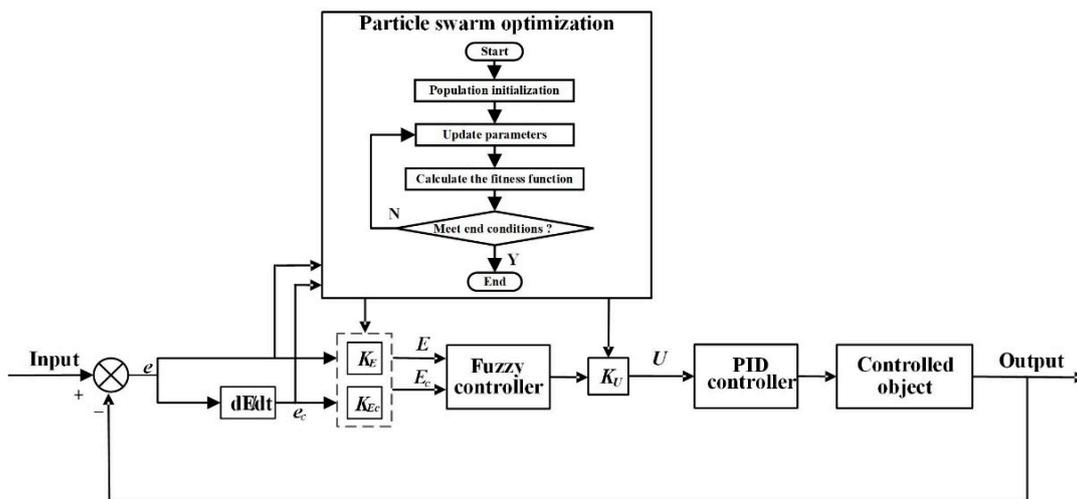
Figure 10. Schematic of fuzzy PID control based on PSO.
