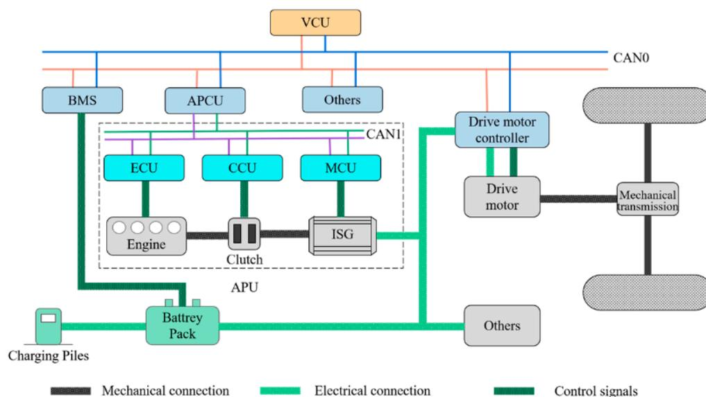
**Figure 2.** Architecture of the whole vehicle's control system.
