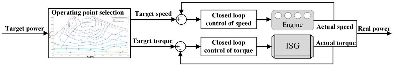
Figure 6. Dual closed-loop coordinated control strategy of APU.
