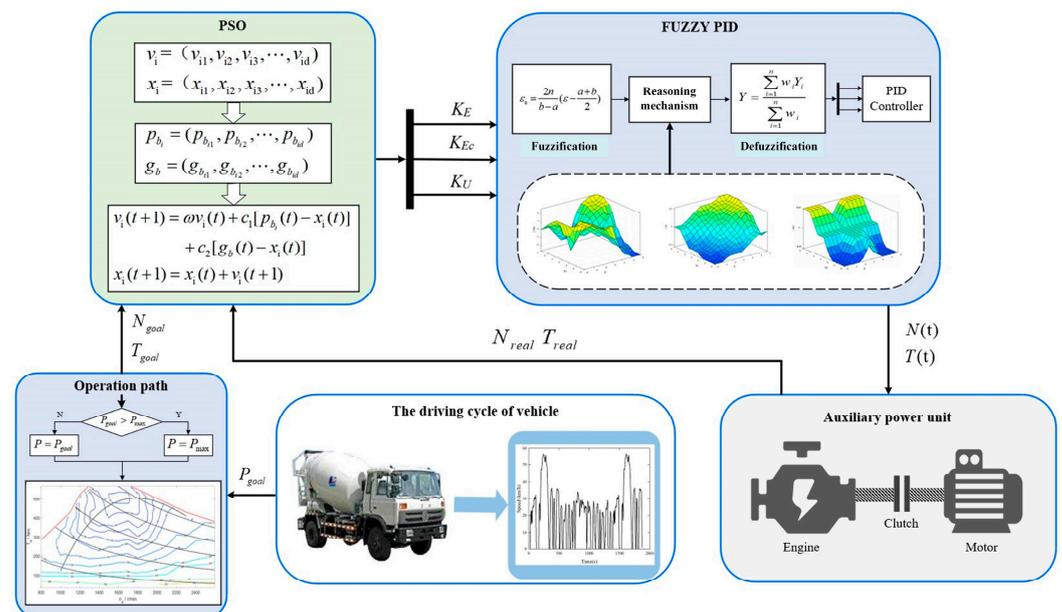
Figure 12. Fuzzy adaptive PID coordination control strategy based on PSO.
