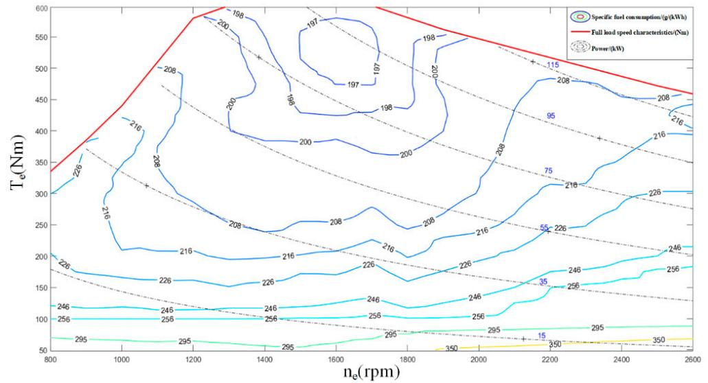
Figure 3. Engine fuel consumption map.
