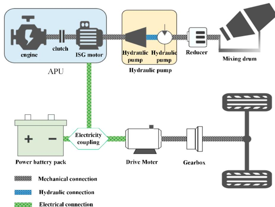
**Figure 1.** Powertrain of extended-range concrete mixer truck.
