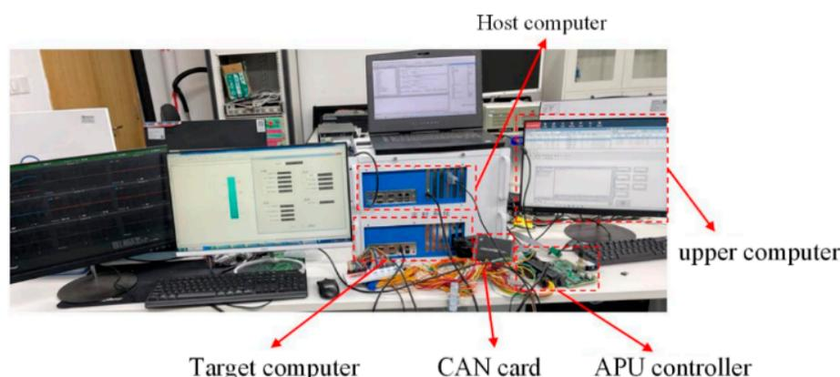
Figure 13. HIL test platform.
