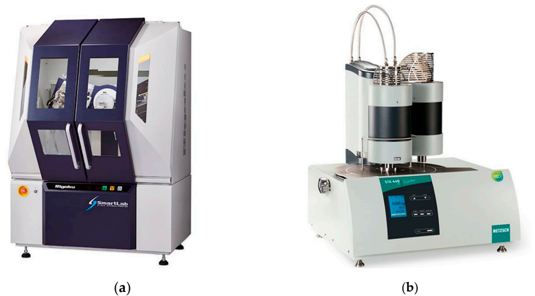
Figure 3. Equipment for mineral composition and differential thermal analysis. (a) is the X-ray diffractometer; (b) is the thermogravimetric analyzer.
