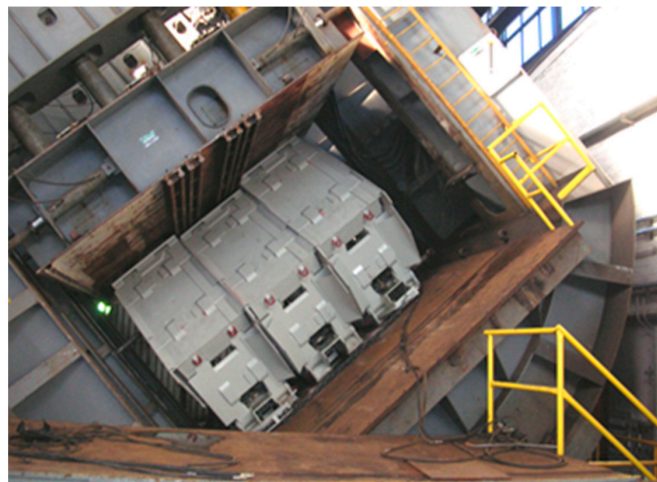
Figure 3. The stand for testing the powered roof supports in KOMAG [19].
