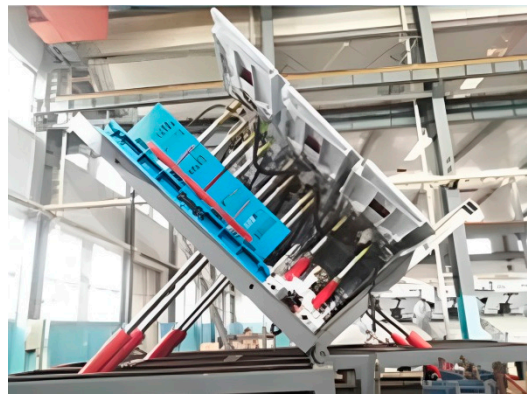
Figure 2. Test for lateral correction force of powered roof supports [18].
