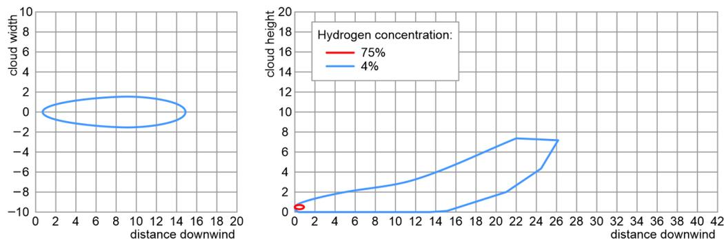
Figure 6. Hydrogen cloud released from a trailer (hydrogen mass: 100 kg, pressure: 20 MPa).
