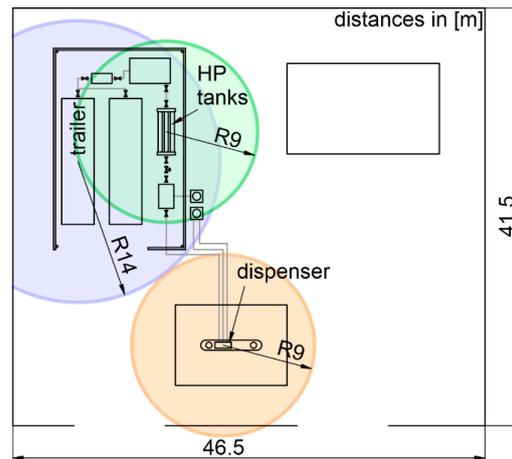
**Figure 15.** Hazard areas where overpressure may cause human death (ignition at the point of hydrogen release).
