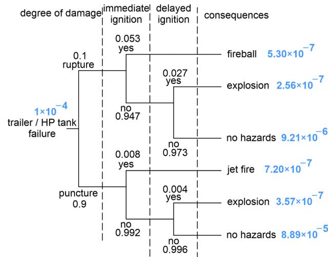
Figure 18. Event tree for a hydrogen release from a trailer or an HP tank.
