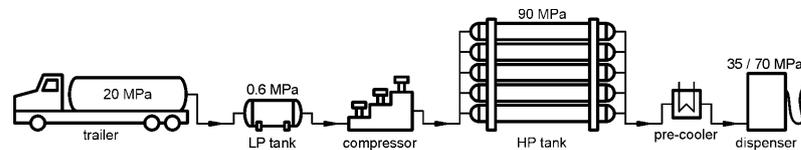
Figure 4. Pressure in the structures of the hydrogen station.
