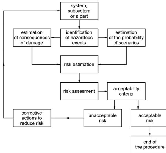
Figure 3. Scheme of the risk analysis procedure.
