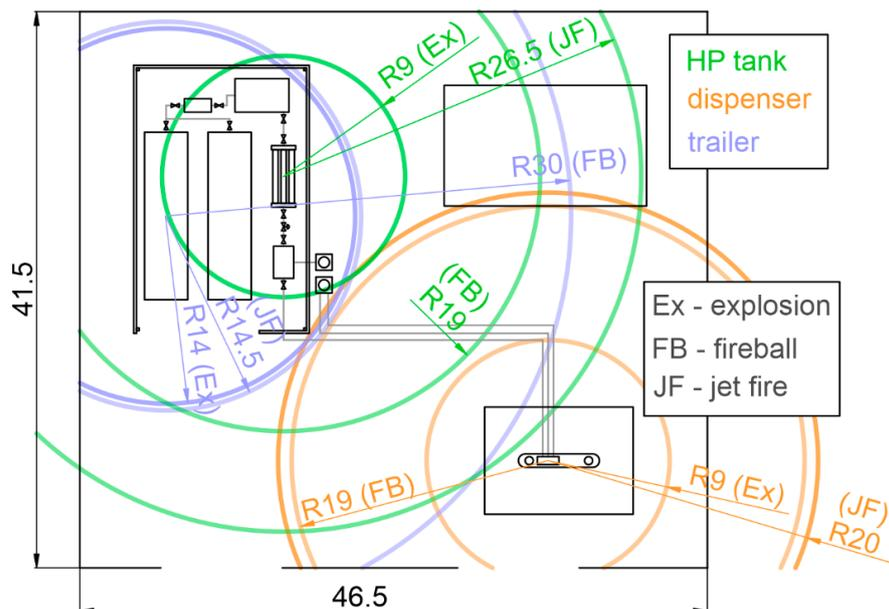
Figure 20. Hazard zones in refueling station after the relocation of the dispenser.
