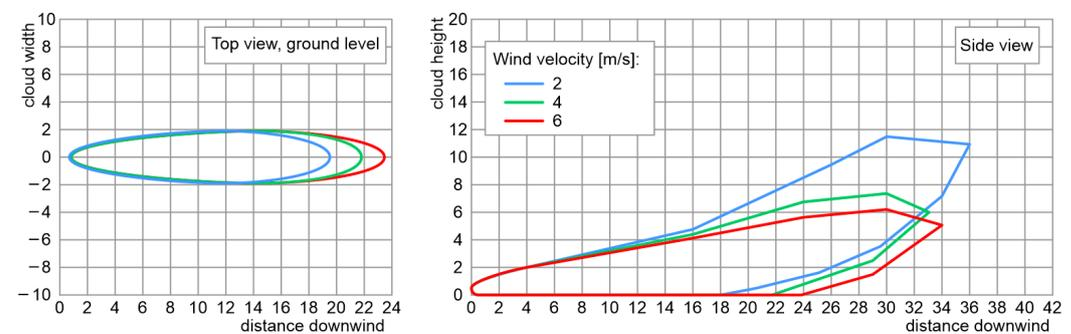
**Figure 10.** Hydrogen cloud released from a dispenser for different wind velocities (hydrogen mass: 25 kg, pressure: 35 MPa).
