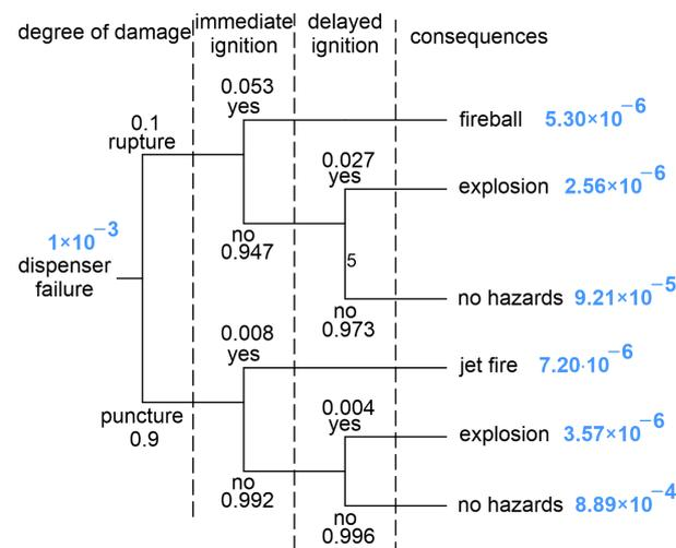
Figure 17. Event tree for a hydrogen release from a dispenser.
