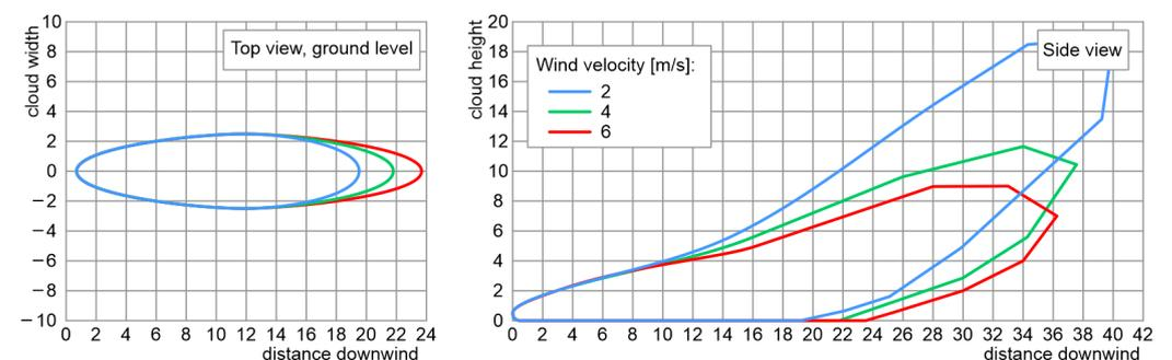
**Figure 11.** Hydrogen cloud released from an HP tank for different wind velocities (hydrogen mass: 25 kg, pressure: 90 MPa).
