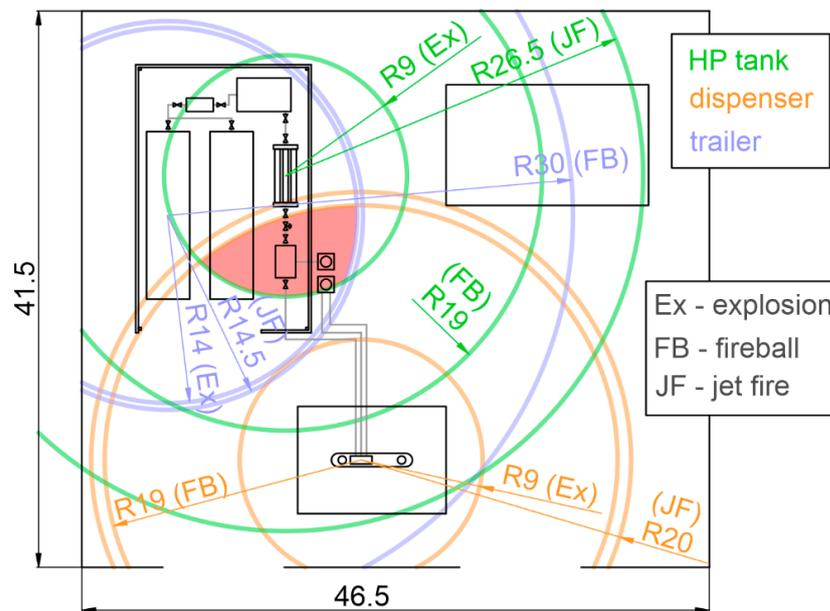
Figure 19. Hazard zones related to fires and explosions of hydrogen released from a trailer, a dispenser or an HP tank (dimensions in meters) with the area of the highest risk marked in red.
