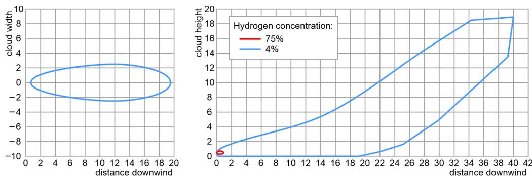
Figure 8. Hydrogen cloud released from an HP tank (hydrogen mass: 25 kg, pressure: 90 MPa).
