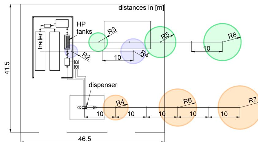
**Figure 16.** Hazard areas where overpressure may cause human death (ignition at a given distance from the point of hydrogen release).
