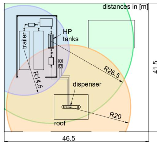
**Figure 13.** Hazard areas where heat flux may cause human death (jet fire).
