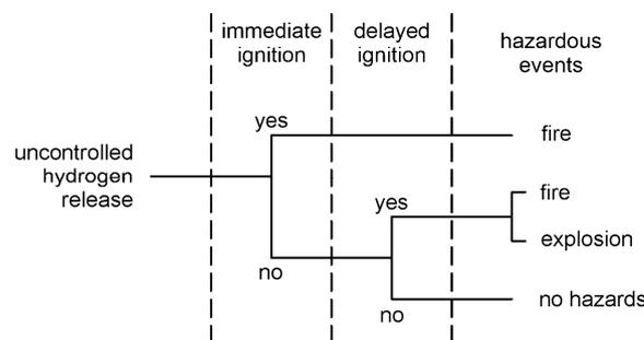
Figure 5. Event tree analysis for the uncontrolled release of hydrogen.
