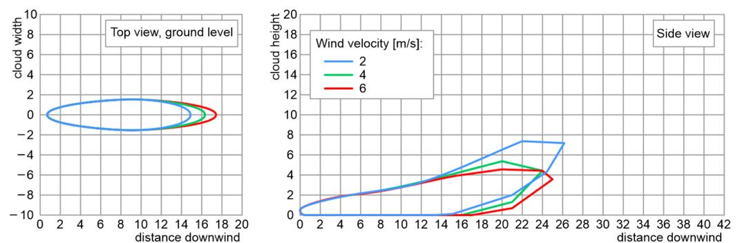
**Figure 9.** Hydrogen cloud released from a trailer for different wind velocities (hydrogen mass: 100 kg, pressure: 20 MPa).
