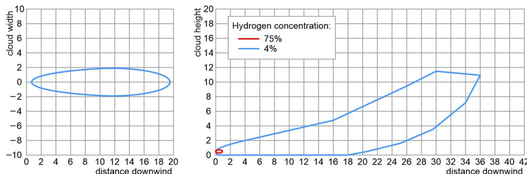
Figure 7. Hydrogen cloud released from a dispenser (hydrogen mass: 25 kg, pressure: 35 MPa).
