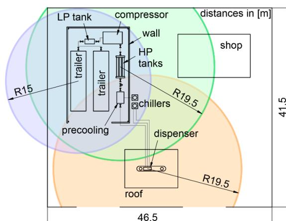
**Figure 12.** Areas of hydrogen concentration above the lower flammability limit (wind velocity 2 m/s).
