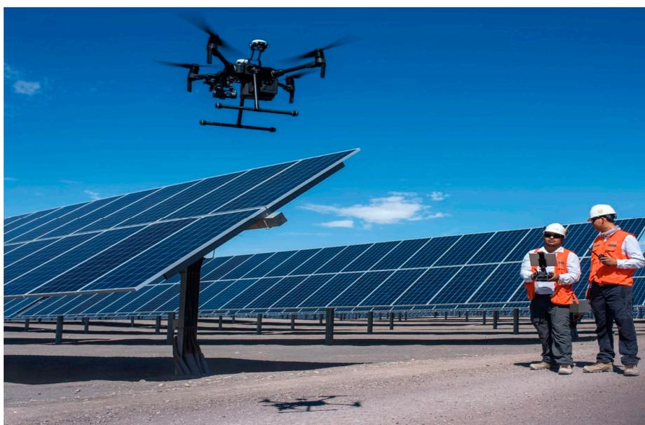
**Figure 33.** An example showing the use of UAVs to detect anomalies in the panels of solar PV farms.
