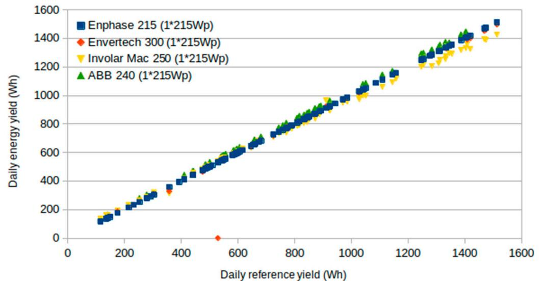
**Figure 10.** Electrical energy yields of different inverters for single PV modules, each connected to a single 215 W<sub>p</sub> module. The daily reference yield (x-axis) is the energy yield (AC) achieved by an Enphase M 215 inverter with a single 215 W<sub>p</sub> module attached.
