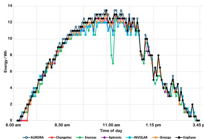
**Figure 7.** Actual recorded data of AC energy generation (over integrals of 5 min) for seven microinverters during the day on 31 October 2013.
