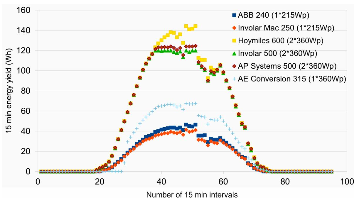
**Figure 9.** Example of electrical energy yield measurements (during intervals of 15 min) of different inverters and two different PV module sizes during a mostly clear day (some clouds in the afternoon).
