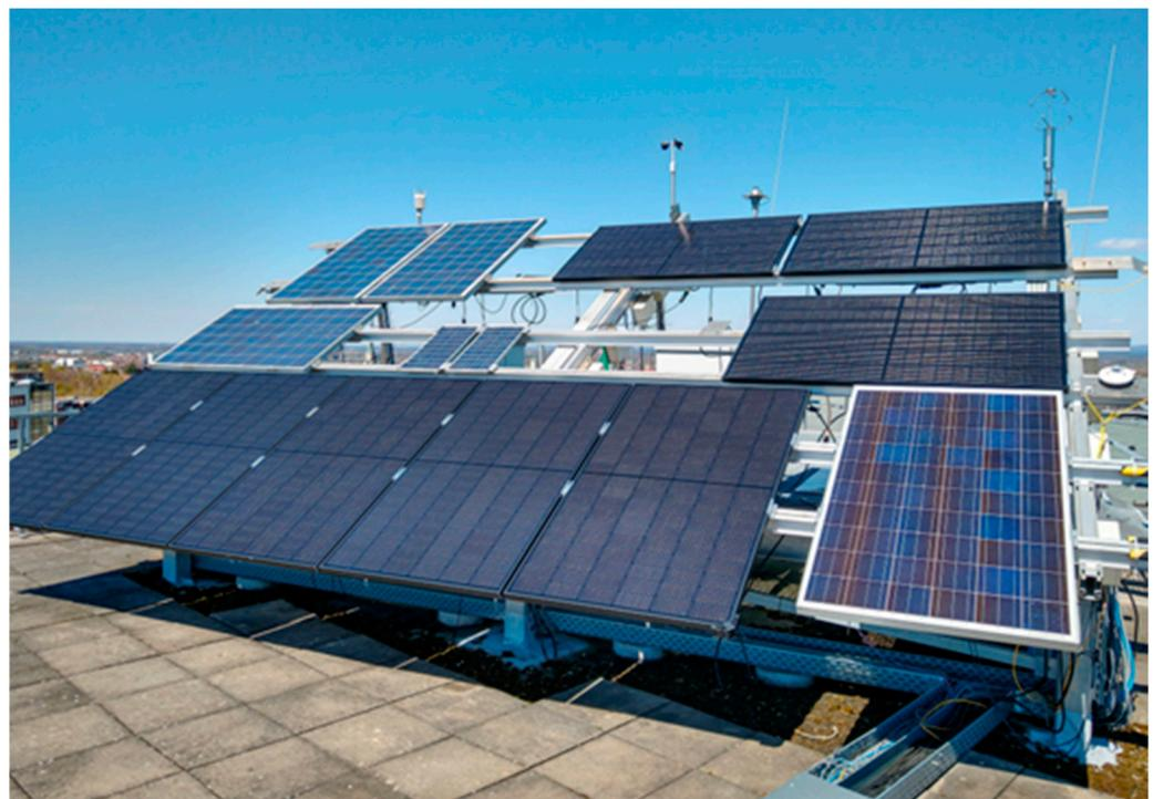
**Figure 4.** Layout of the PV modules of the PV outdoor laboratory in 2023 for the electrical energy yield comparison of microinverters using eight to ten equal, calibrated PV modules (of  $360 W_p$  each) as inputs.
