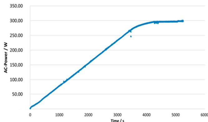
**Figure 2.** Measured AC power output (in Watts) as a function of measurement duration (in seconds) for a linear increasing DC input current for a 300 W inverter.
