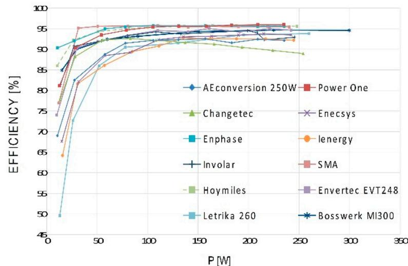
**Figure 5.** Measured DC–AC conversion efficiencies as a function of power outputs for 12 microinverters with single PV module inputs.
