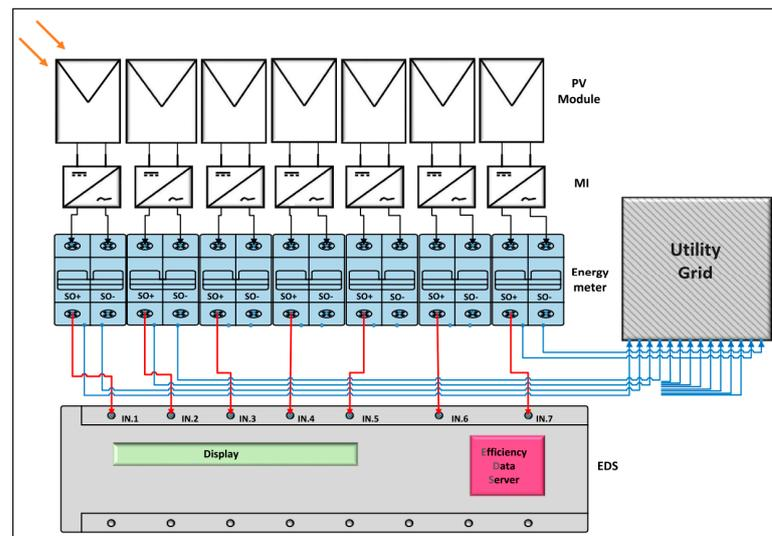
**Figure 3.** Outdoor measurement setup for the microinverters (MIs).
