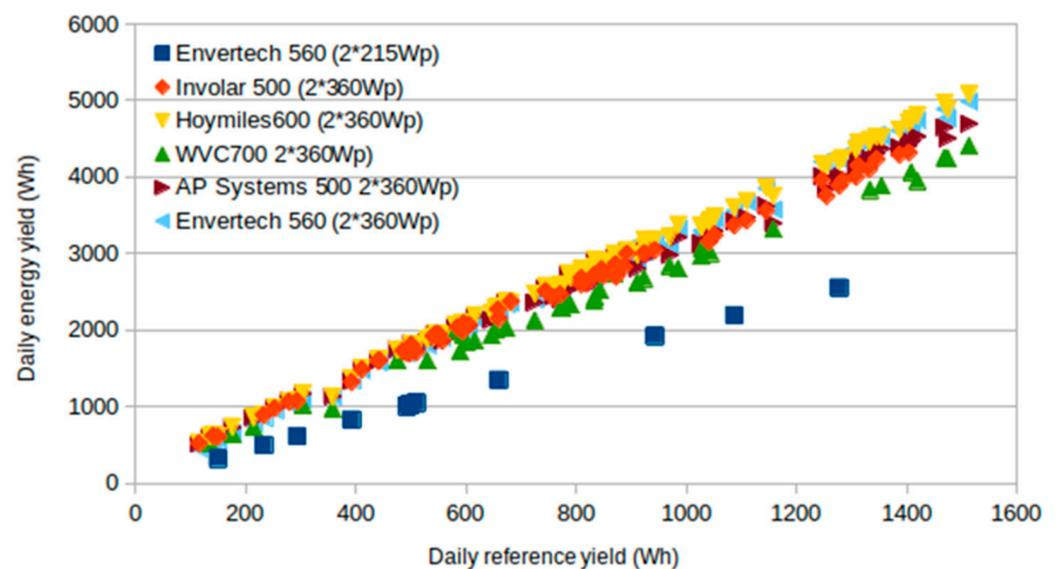
**Figure 11.** Average daily energy yields (AC) of different inverters for two modules with two 215 W<sub>p</sub> or 360 W<sub>p</sub> modules attached. The reference yield (*x*-axis) is the yield achieved by an Enphase M 215 with a single 215 W<sub>p</sub> module applied.
