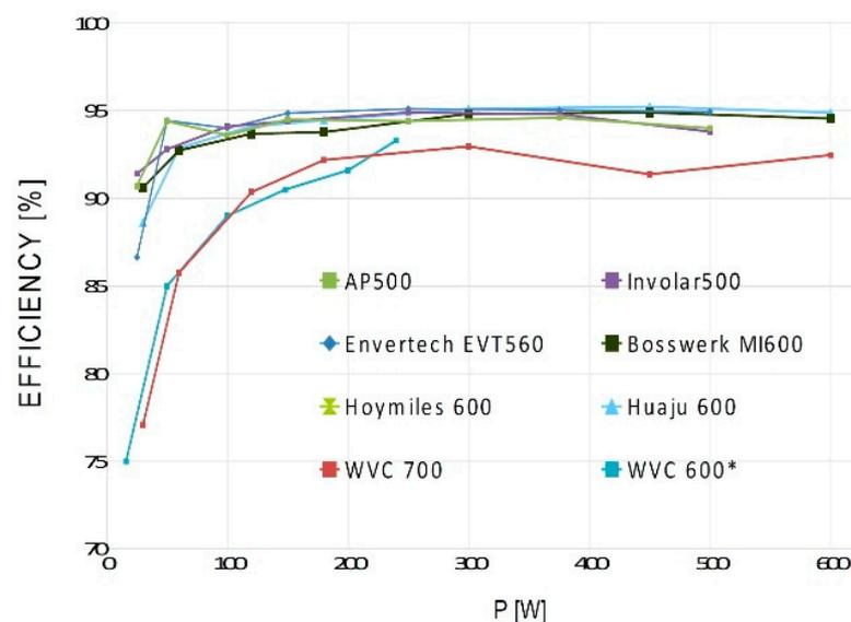
**Figure 6.** Measured DC–AC conversion efficiencies as a function of power outputs for eight microinverters with two PV module inputs. \* failed.
