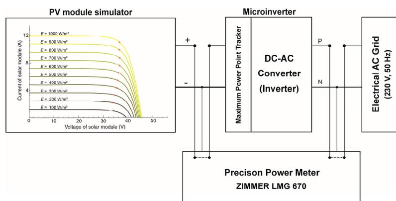
**Figure 1.** Setup of the indoor power and efficiency measurements using a black box approach via utilising a precision power metre for inputs and outputs.
