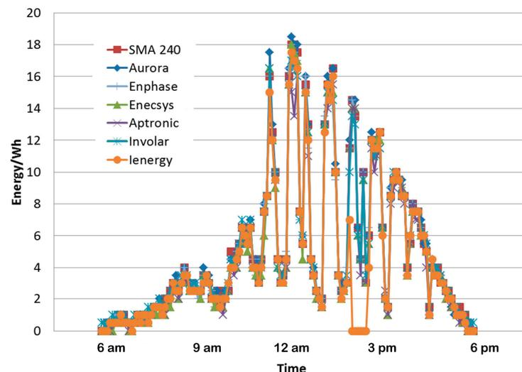
**Figure 8.** Actual recorded data of AC energy generation of seven microinverters (over integrals of 5 min) during the day on 6 April 2015.
