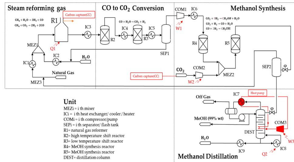
Figure 4. Process flow diagram of proposed MeOH production plant simulated in HYSYS (ALT 1-ALT4).
