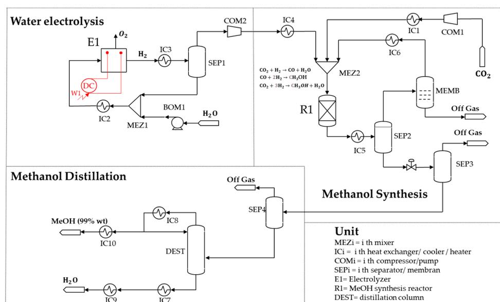
Figure 1. Process flow diagram of a “green” methanol production by electrolysis (ALT5).
