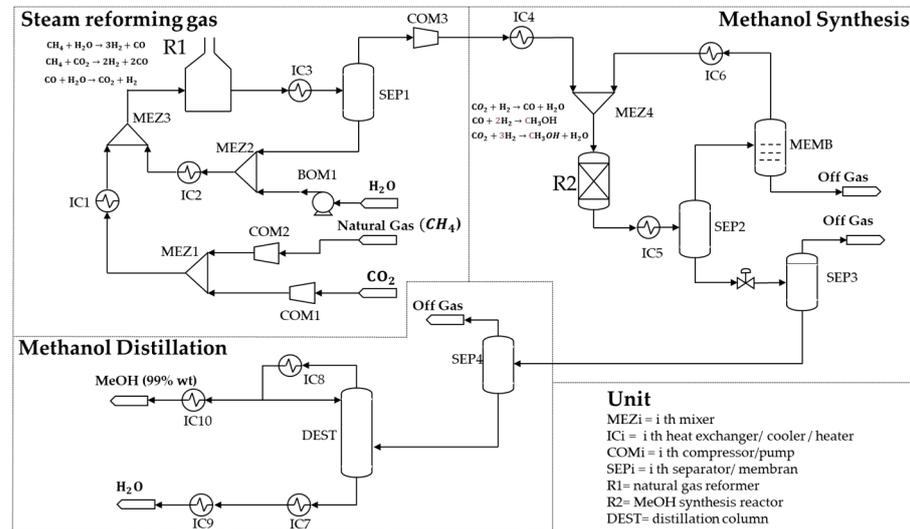
Figure 3. Process flow diagram of MeOH production plant simulated in HYSYS—base case.
