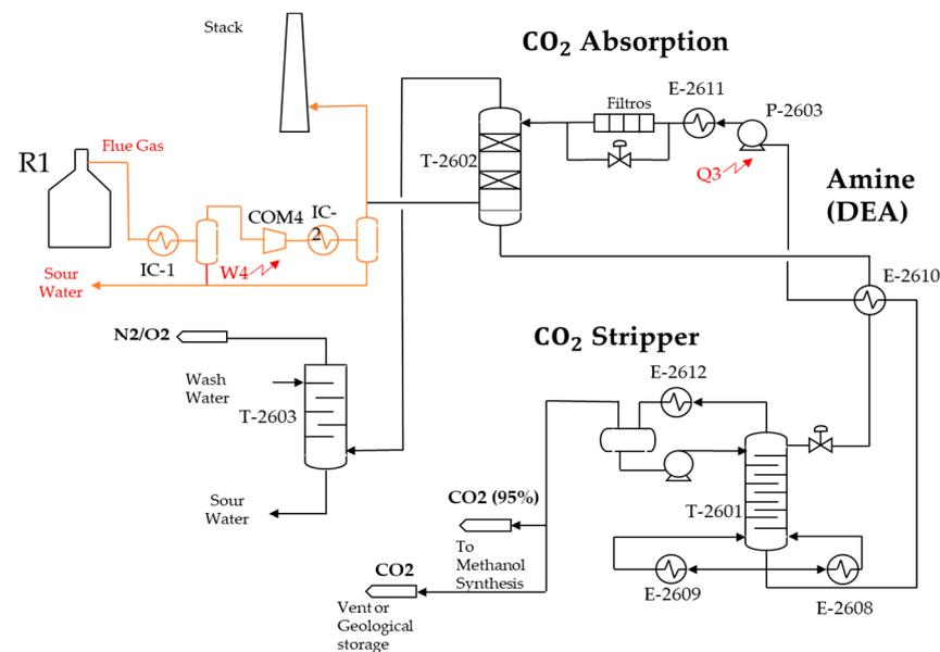
Figure 6. Process flow diagram of the existing carbon capture unit (CCU) based on DEA absorption (for Base, ALT 1 to ALT 3) (orange lines indicate changes required).
