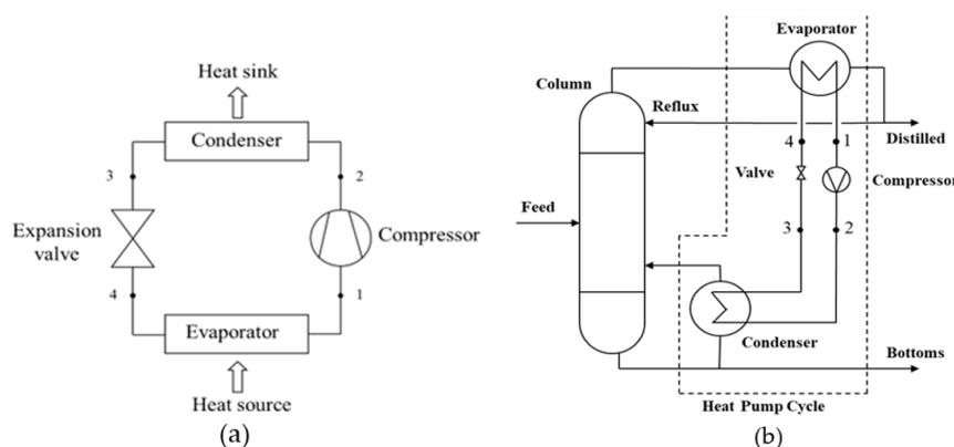
**Figure 2.** (a) Schematic diagram of the heat pump system and (b) application of the heat pump in the distillation column.
