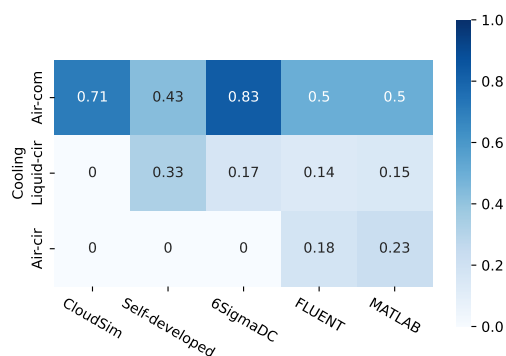
Figure 4. Heatmap of three cooling indicators on five simulators, ordered by the comprehensive ability of cooling simulation.
