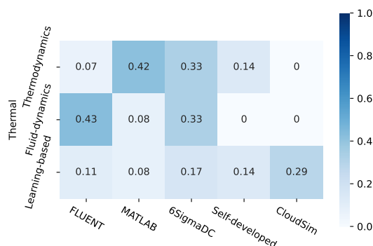
Figure 7. Heatmap of three thermal indicators on five simulators, ordered by the comprehensiveness of thermal model.
