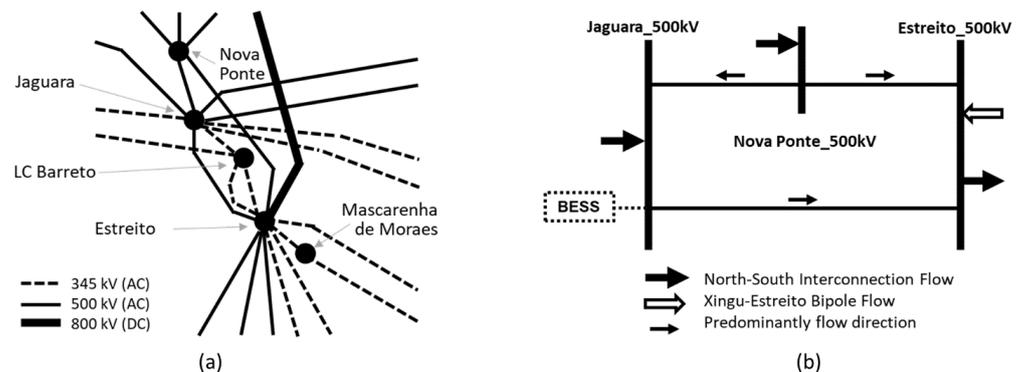
**Figure 6.** (a) Part of the NMG electric grid; (b) One-line diagram of the Jaguará, Nova Ponte, and Estreito substation connections.
