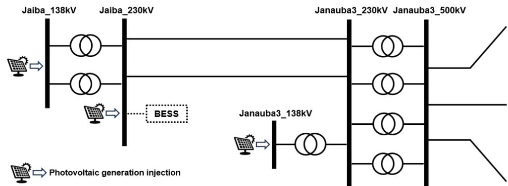
**Figure 5.** Jaiba and Janauba substations electric connections.
