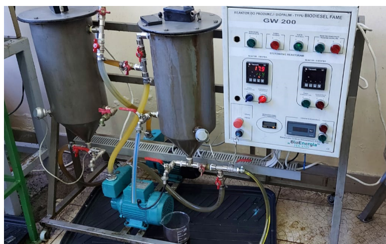
Figure 2. Photo of the GW200 reactor used for ester production (Malopolskie Center of Renewable Energy Sources “BioEnergia”, Krakow, Poland).
