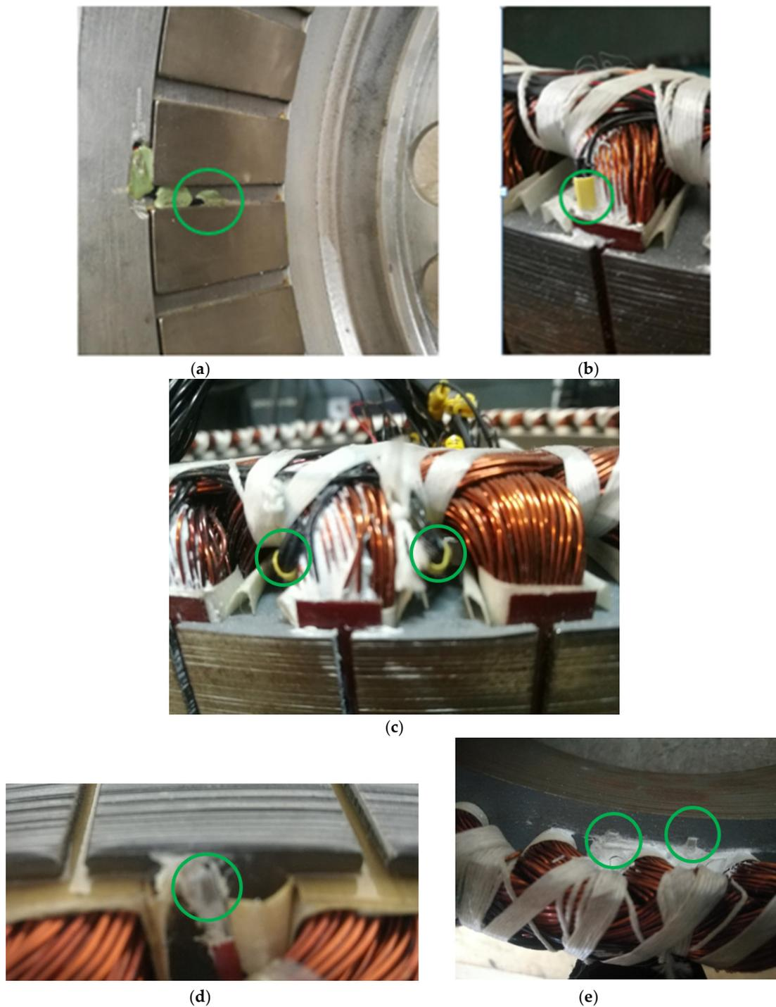
**Figure 9.** Arrangement of temperature sensors: (a) on the magnet, (b) in the slot (top of the slot), (c) temperature sensor terminals from the winding fronts, (d) temperature sensor terminals from the stator core (top of the tooth) and (e) stator core temperature sensor (bottom of the tooth/stator yoke).
