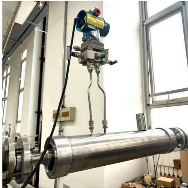
Figure 6. Photograph of the perforated plate flowmeter.
