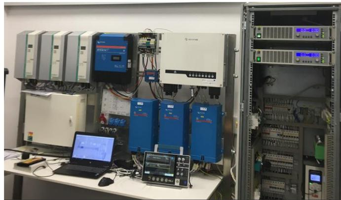
**Figure 13.** Test stand designed for testing grid-tied inverters.
