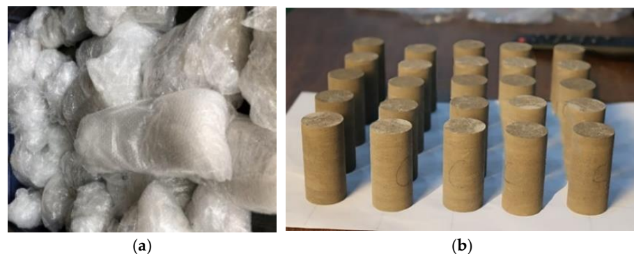
Figure 1. Original rock and prepared mudstone samples. (a) Original rock from Liangjia Coal Mine; (b) prepared mudstone samples.
