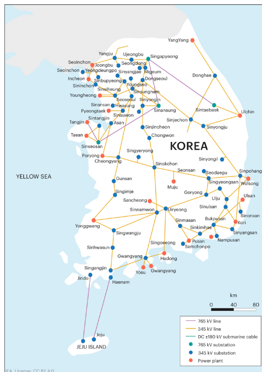
Figure 2. Power grid system of South Korea (cited from International Energy Agency, available at https://www.iea.org/articles/korea-electricity-security-policy (accessed on 28 April 2024).
