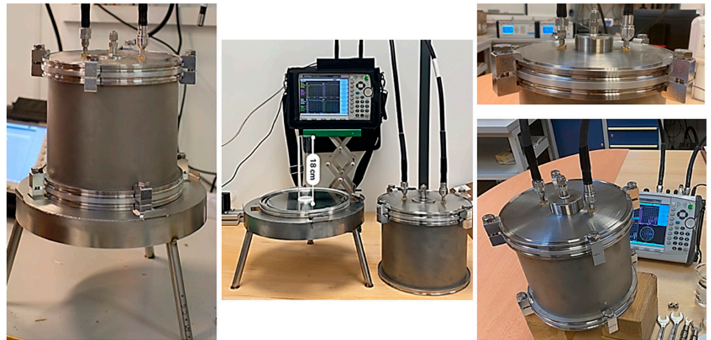
Figure 8. The electromagnetic resonant cavity.
