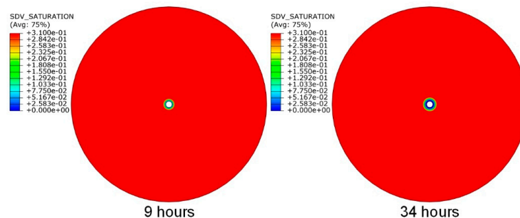
Figure 9. Changes in hydrate saturation after wellbore opening.
