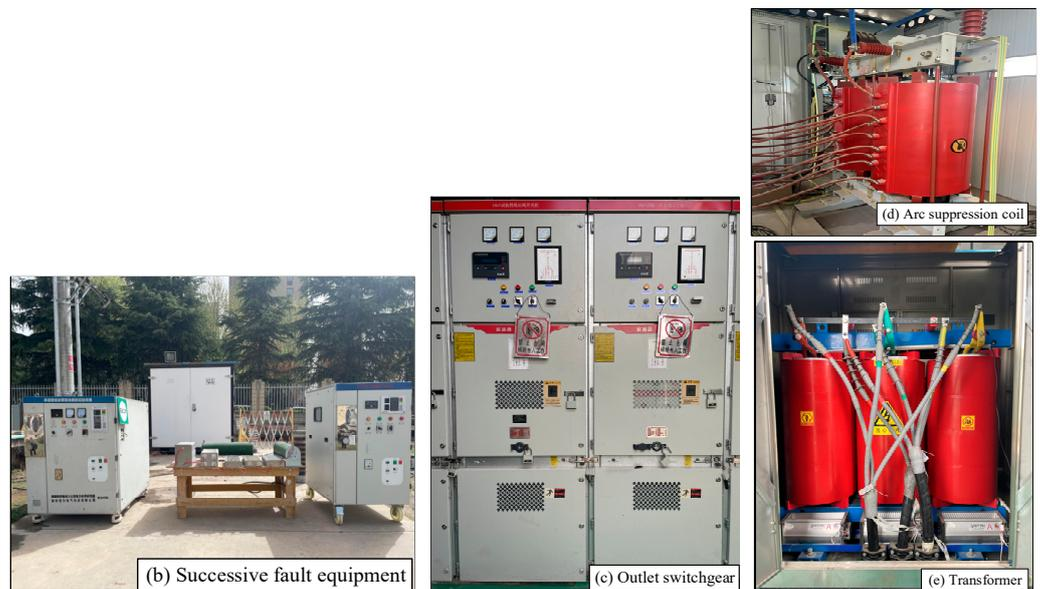
Figure 16. The 10 kV full-scale test field wiring.
