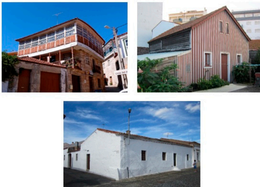
Figure 3. (above, left) A three-story stone house with glazed balconies to improve solar gains, in Salzedas, North Portuguese region; (above, right) wooden hut in Mira Beach, on the country’s central coastline; (below) an earthen single-story house in Moura, in the southern region of Alentejo. Reproduced with permission from Jorge Fernandes.
