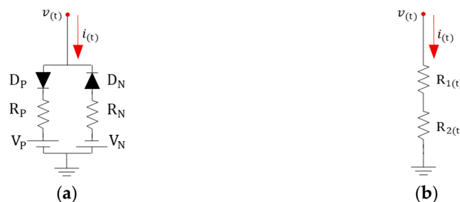
Figure 8. High impedance fault models: (a) based on active and passive circuit elements; (b) based on passive circuit elements.
