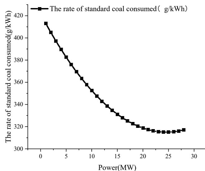
**Figure 5.** Standard coal consumption characteristics of the generator set.
