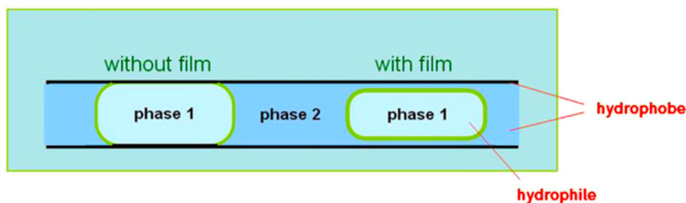
Figure 15. Gas slug surrounded with a liquid film in between the gas slug and microchannel capillary wall [82].
