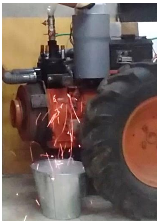
Figure 11. Biomass-fueled engine prototype idling.
