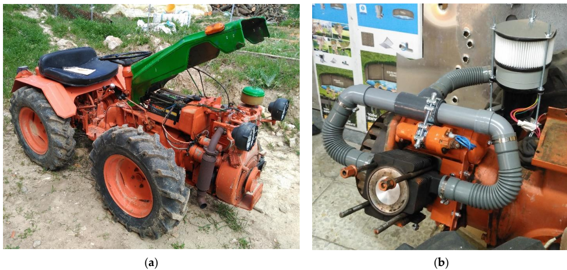
Figure 2. (a) Base engine fitted in the tractor; (b) engine with the modified cylinder and piston. The blower with the air filter is placed at the top right.
