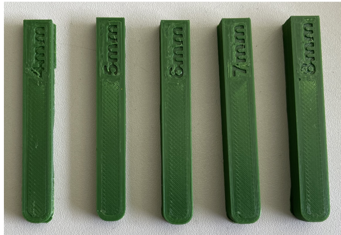
Figure 5. The 3D-printed-spacers used during experiments to perform gap length adjustments.
