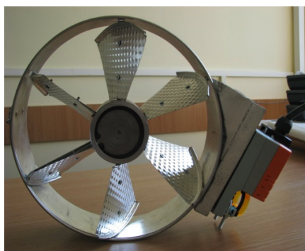
Figure 4. A two-flow air diffuser (TFAD), equipped with electric actuator Belimo LM24A.
