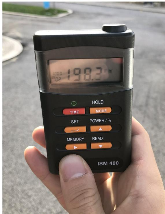
**Figure 14.** Illustration of the horizontal irradiance acquisition taken on the roof and near the two modules periodically.
