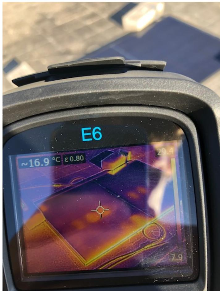
**Figure 15.** Picture of the thermographic camera used to measure and visualize the temperature distribution through the PERC and HJT modules.
