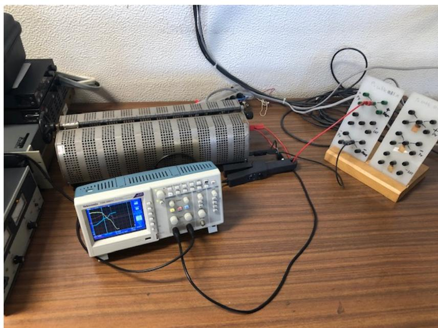
**Figure 12.** Photo of the system used to analyze the voltage and electric current signals from the HJT and PERC panels. Above the oscilloscope image, the electrical resistance connected to each panel, HJT or PERC, is shown.
