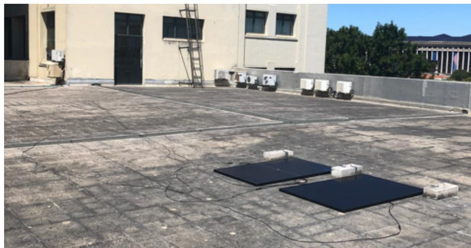
**Figure 10.** Expanded roof view of the HJT and PERC modules and their cable connections to our laboratory.
