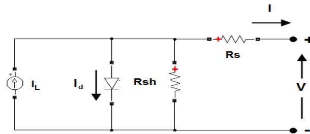
Figure 7. Circuit diagram of the PV array [36].
