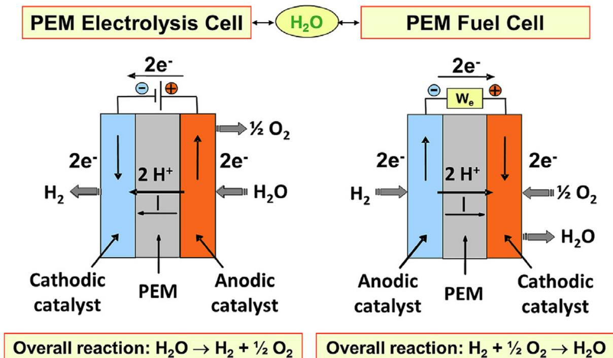
Figure 1. Chemical reactions of a PEM electrolyzer [8].
