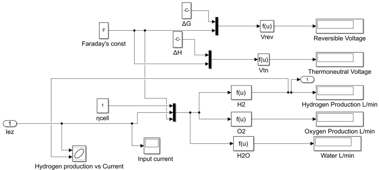
Figure 12. Simulink model of a PEM electrolyzer.
