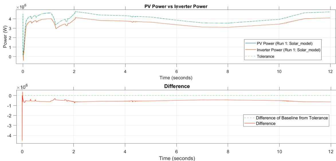
Figure 16. Comparison between PV and inverter output.
