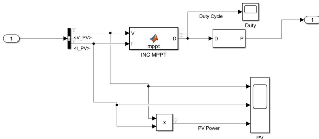
**Figure 6.** MPPT model with duty cycle for regulating PV's varying voltage.
