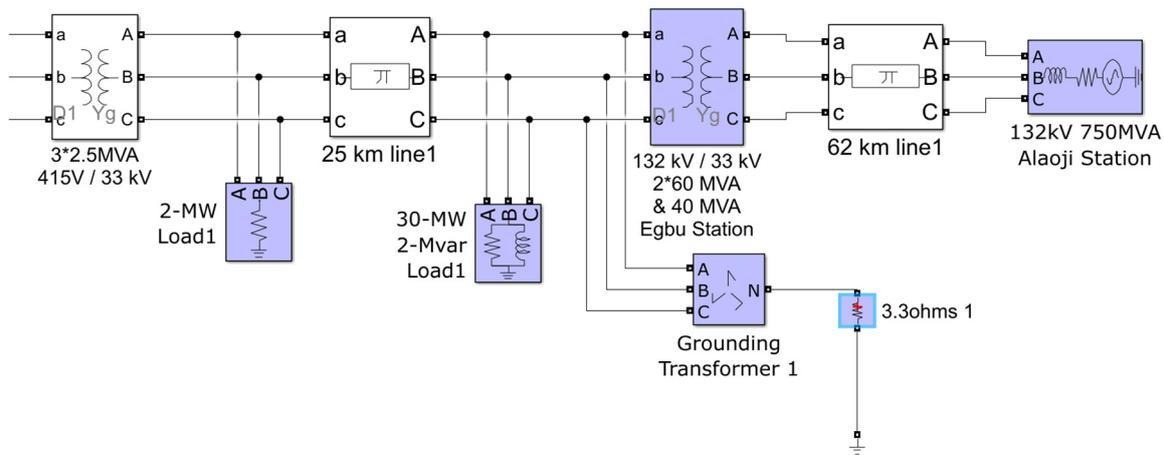
Figure 11. Simulink model of Owerri 132/33 KV transmission station.
