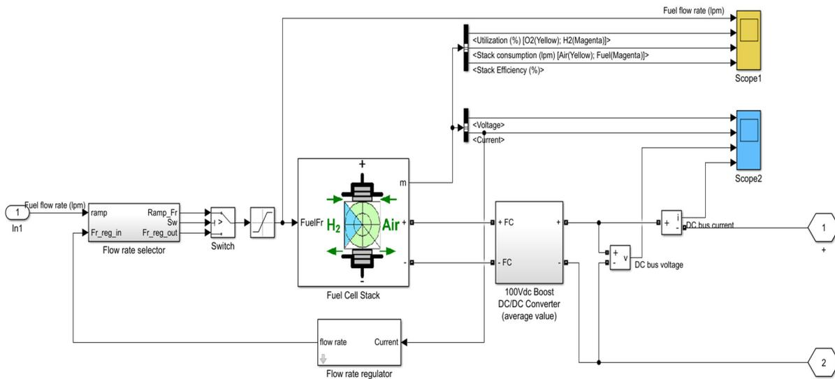
Figure 14. Dynamic model of the fuel cell system.
