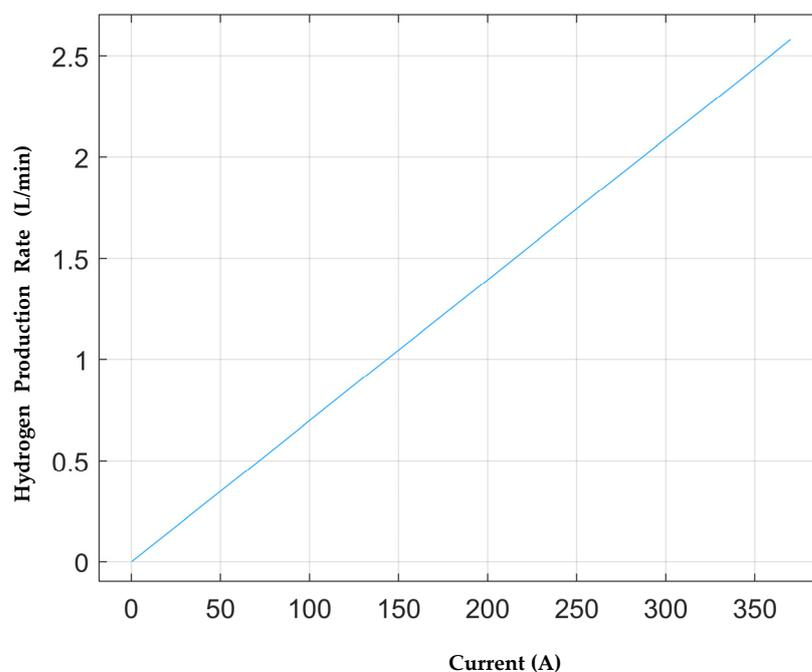
Figure 17. Graph of hydrogen production rate vs. electrical current.
