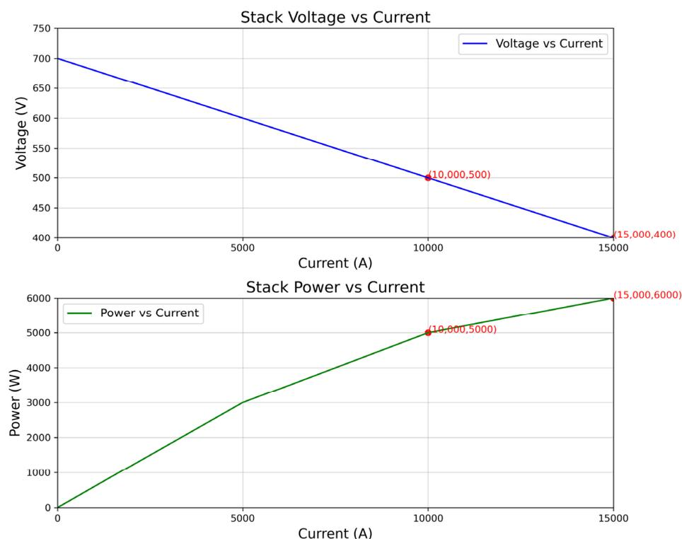
**Figure 18.** The 5 MW fuel cell power, voltage, and current. The fuel cell with the PV–wind turbine system supplies the needed power despite varying irradiance and wind speed.
