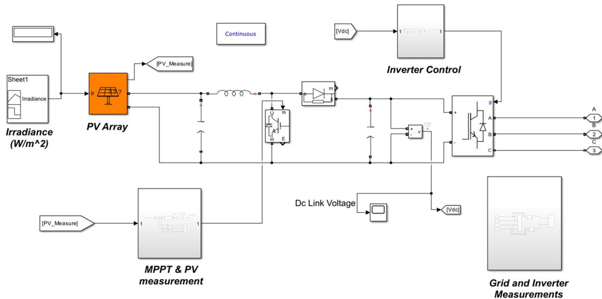
Figure 8. PV generator connected to a buck DC converter and an inverter.
