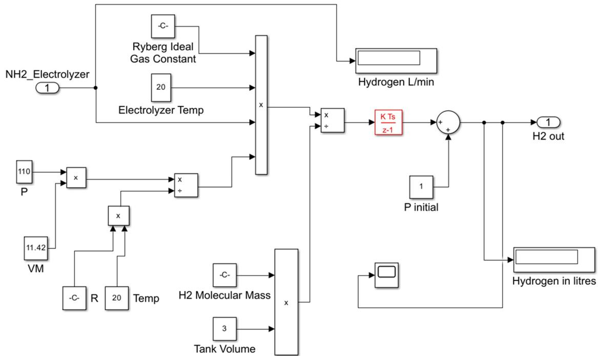
Figure 13. Simulink model of a PEM electrolyzer tank.
