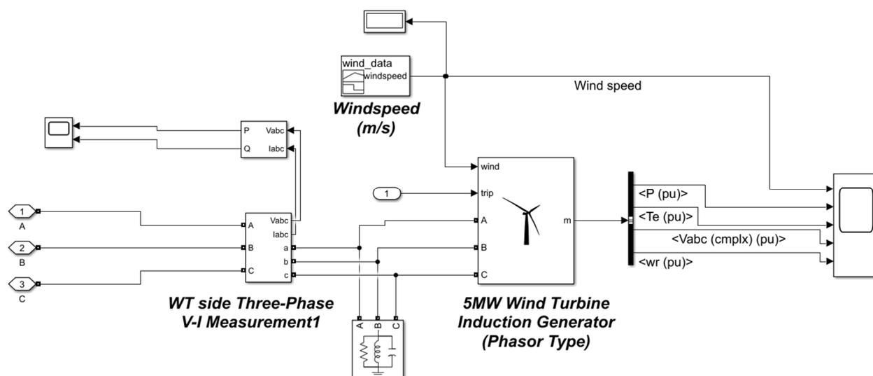
Figure 10. Wind turbine and induction generator.
