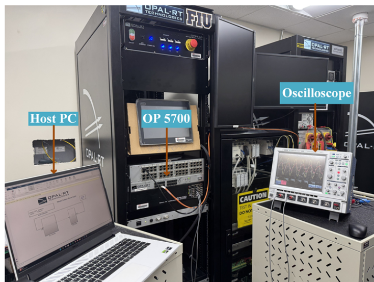
Figure 12. Real-time simulation setup using Opal-rt OP5700.
