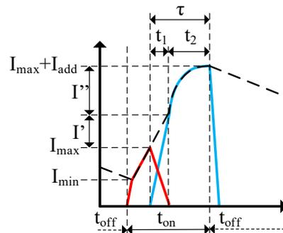
**Figure 9.** A more detailed picture describing the transient processes of the CB discharge. The black dashed curve is the current in the SC circuit; the red curve is the current of the main thyristor; and the blue curve is the current of the CB discharge.
