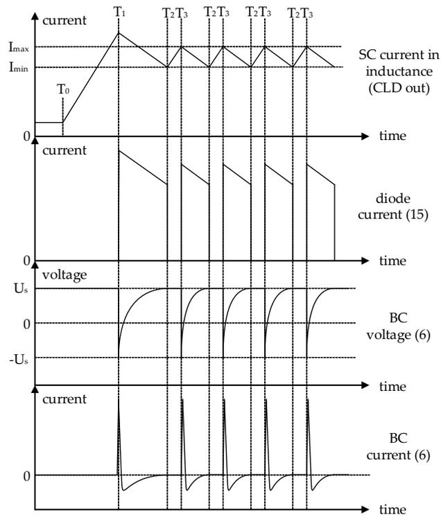
Figure 4. Oscillograms of transient processes during various stages of CLD operation.
