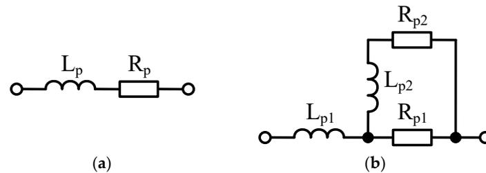
**Figure 14.** The equivalent circuit of the electromagnetic reactor of the DC circuit: (a) excluding the influence of skin effect and proximity effect; (b) taking into account the influence of the skin effect and the proximity effect.
