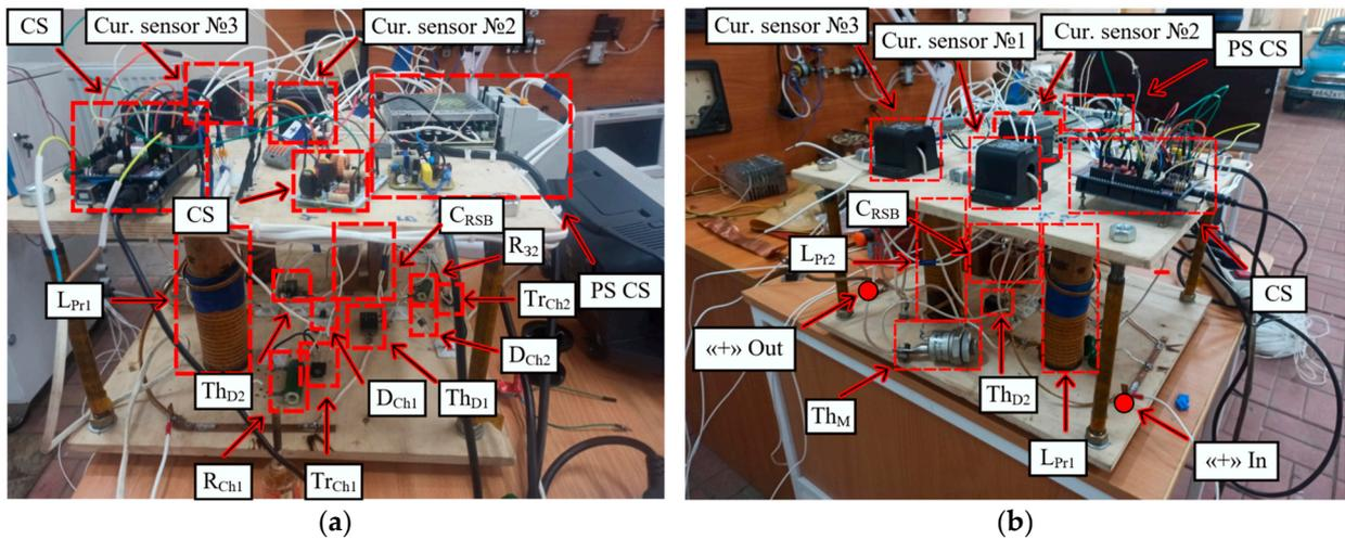
**Figure 10.** Appearance of the created prototype of the current-limiting device. (a) Photograph, view 1. (b) Photograph, view 2.
