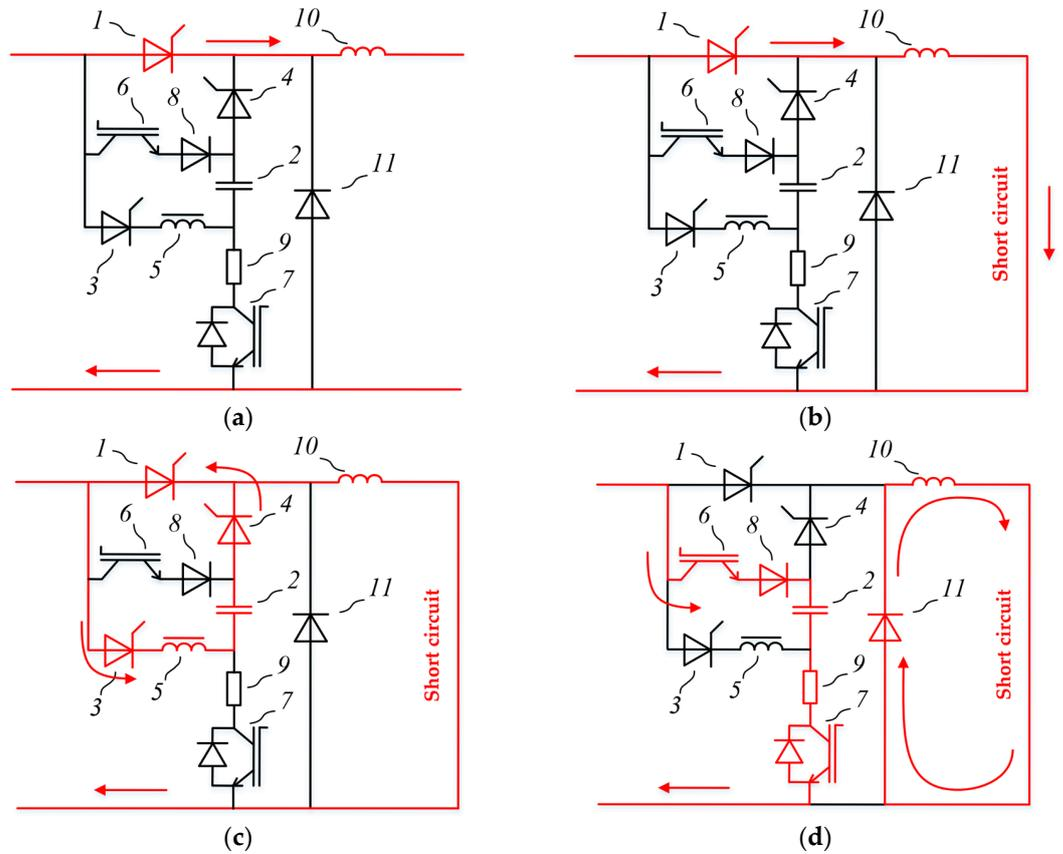
Figure 5. The stages of operation of the current-limiting device. (a) Nominal operation mode (time interval  $0-T_0$  in Figure 4). (b) The occurrence of a short circuit or the activation of the main thyristor (time intervals  $T_0-T_1$  or  $T_2-T_3$ , respectively, in Figure 4). (c) The artificial switching of the thyristor (time moment  $T_1$  in Figure 4). (d) The current pause of the CLD (time intervals  $T_1-T_2$  and  $T_3-T_2$  in Figure 4).
