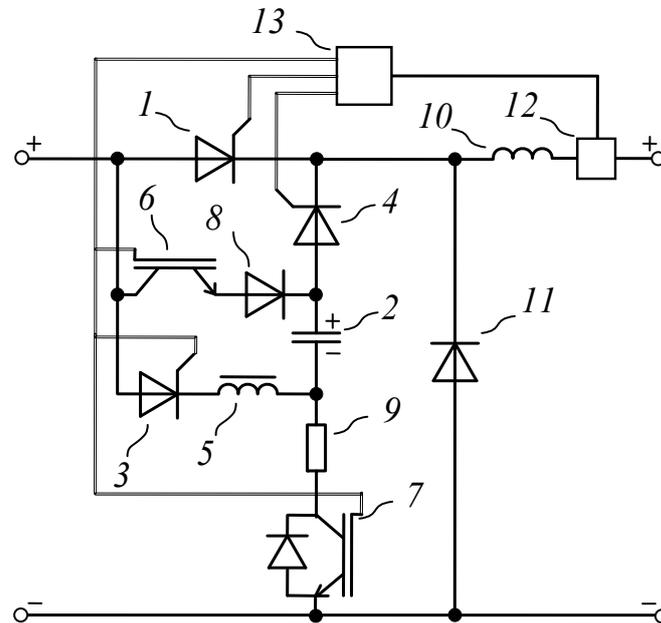
**Figure 3.** Electrical diagram of a semiconductor current-limiting device.
