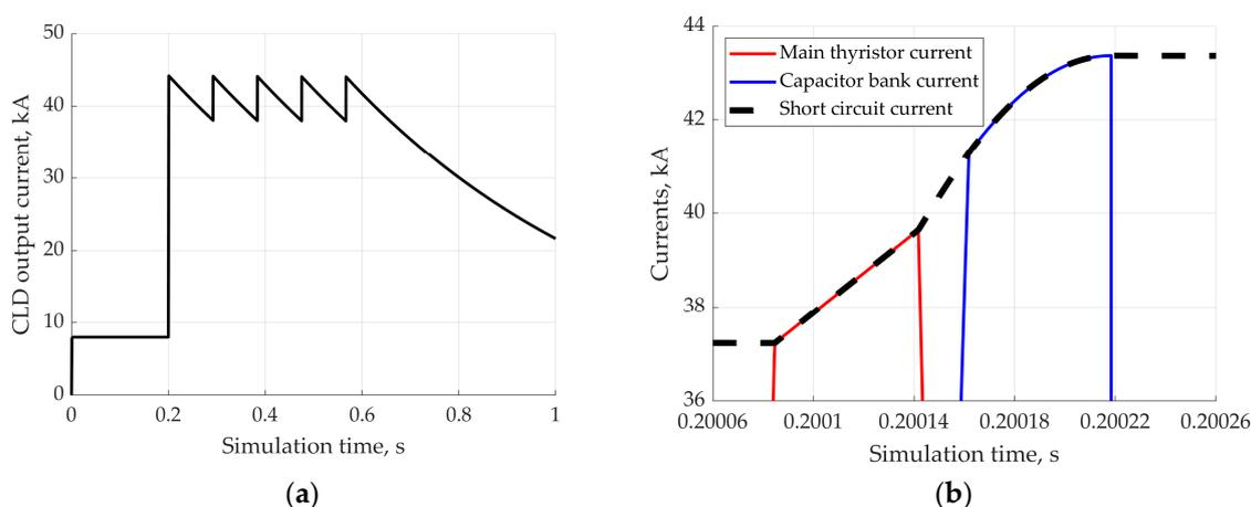
**Figure 16.** The simulation results of a powerful prototype of a current-limiting device. (a) The output current of the current-limiting device. (b) The transients in the CLD at the time of artificial switching of the thyristor and the CB discharge.
