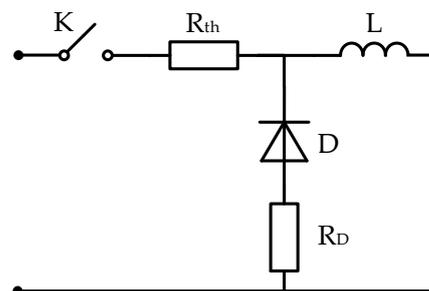
Figure 6. Current-limiting device equivalent circuit.
