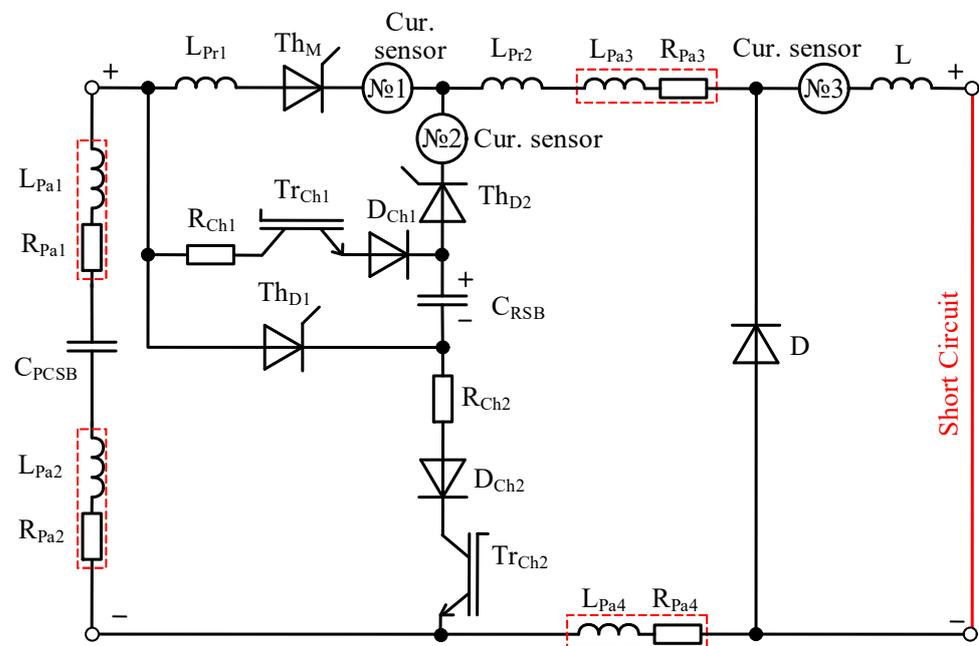
**Figure 11.** An electrical diagram of the experimental setup.
