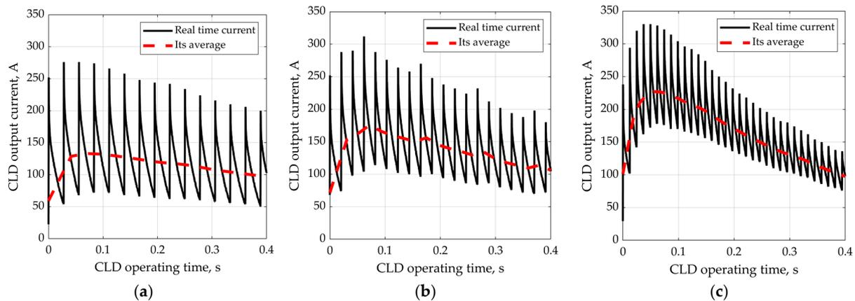
**Figure 12.** The current oscillograms at the CLD output (black solid line denotes experimental results; red dotted line is the average value) at a  $C_{PCSB}$  precharge voltage of 500 V. The CLD operating frequency is (a) 36 Hz; (b) 48 Hz; and (c) 81 Hz.
