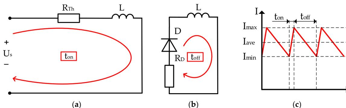
Figure 7. The transients of the current-limiting device: (a) the main thyristor is on; (b) the main thyristor is off; and (c) the current at the output of the current limiter/converter.
