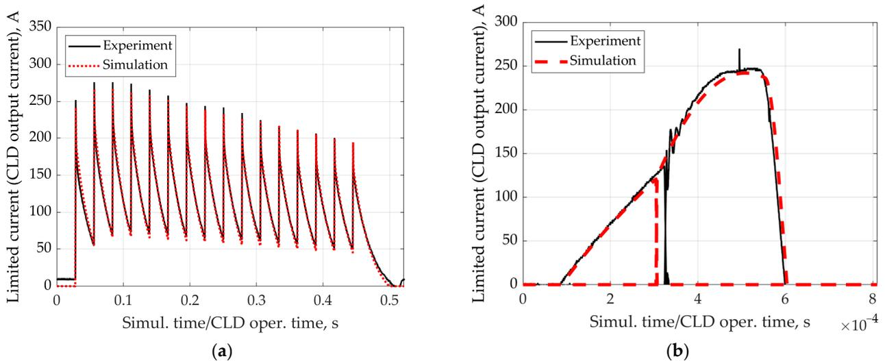
**Figure 15.** A comparison of the computer simulation and experimental results. (a) The output current of the current-limiting device. (b) The transients in the CLD at the time of artificial switching of the thyristor and the CB discharge.
