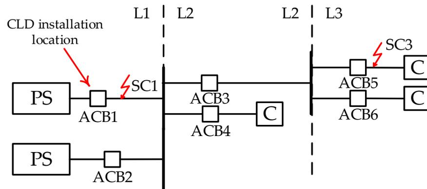
**Figure 1.** Sample diagram of a power system section for clarification of the principle of the selective operation of switching equipment.
