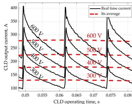
**Figure 13.** The current waveforms at the CLD output (the black solid line denotes the experimental results; the red dotted line is the average value) for the CLD operating at 81 Hz. The  $C_{PCSB}$  precharge voltage is indicated directly at the waveforms.
