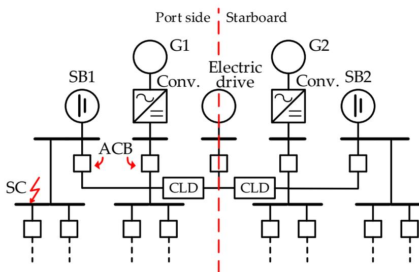
**Figure 2.** A diagram of the power system of a prospective vessel equipped with electric propulsion.
