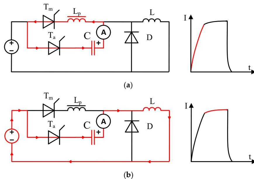
**Figure 8.** The transients of the CB discharge: (a) an approximate view of the substitution scheme and the oscillogram of the current at the output of the CLD, transients of the first stage; (b) transients of the second stage.
