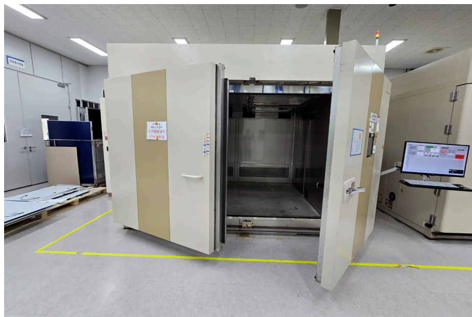
Figure 6. Solar simulator chamber used for tests IEC 61215 and DIN 75220.
