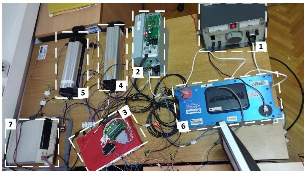
**Figure 16.** HIL simulation emulation setup: 1—autotransformer; 2—Danfoss FC302 converter; 3—Typhoon HIL 402; 4, 5—LiFePO<sub>4</sub> batteries; 6—Maxwell BMOD0083 P048 B01 supercapacitor; 7—Fluke multimeter.
