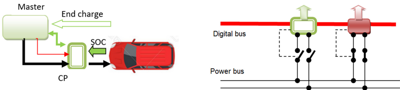
Figure 18. Power supply control scheme at the CP.
