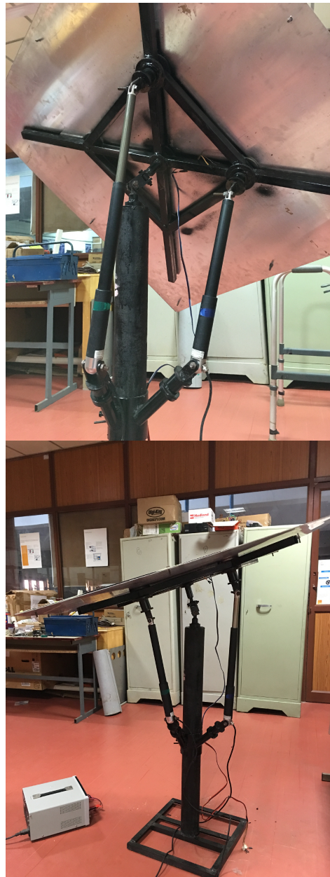
Figure 12. Tilt-Roll heliostat prototype built earlier for inverse kinematics validation [46].
