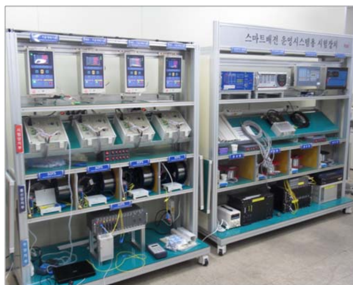
Figure 13. Test devices of automatic fault processing.
