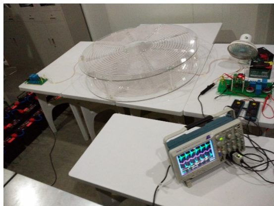
Figure 19. A prototype of a wireless charging system.
