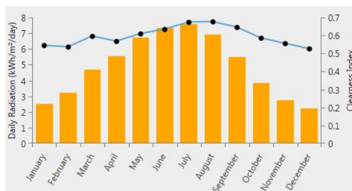
Figure 3. Daily global horizontal solar radiation and clearness index in Andalusia implemented with Hybrid Optimization of Multiple Energy Resources (HOMER) software.
