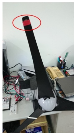
Figure 24. A block attached near the tip of a blade.
