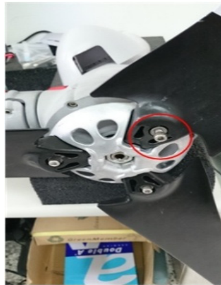
Figure 23. A blade with a loose hug screw.
