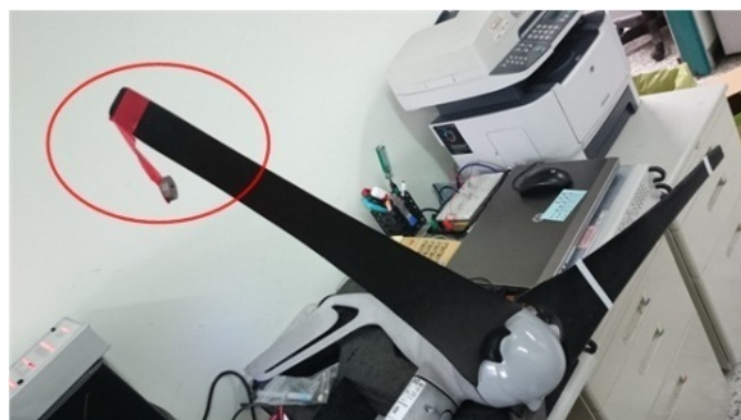
Figure 25. A blade with a hanging mass.
