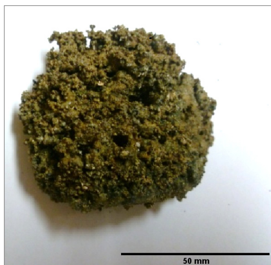
Figure 3. Bed sintering of wood pellet after 3 h of stable combustion.
