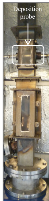
Figure 1. Picture of the experimental facility: a lab-scale low-power biomass combustion boiler. The deposition probe position is indicated.
