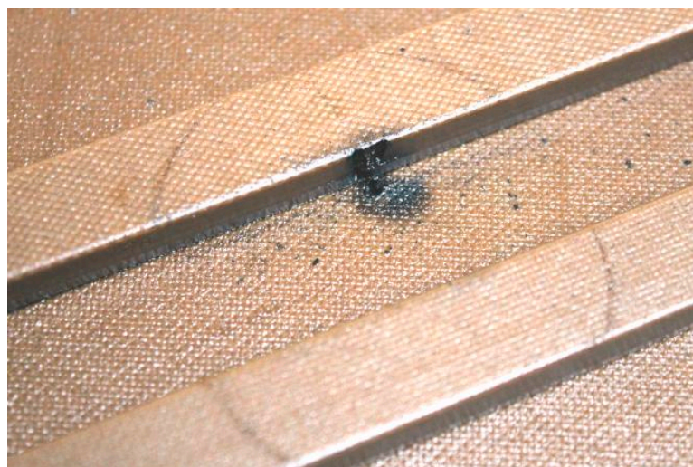
Figure 12. Traces of surface PD on an insulation sample with a moisture content of 5.7%.
