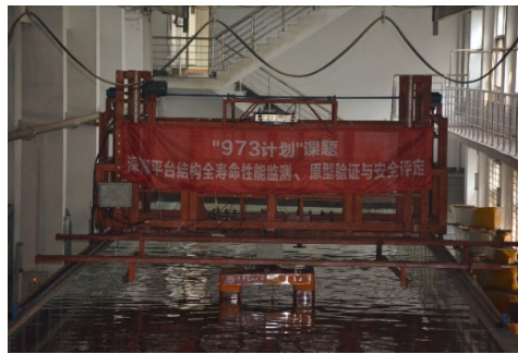
Figure 7. The picture of the scale model in the wave tank.
