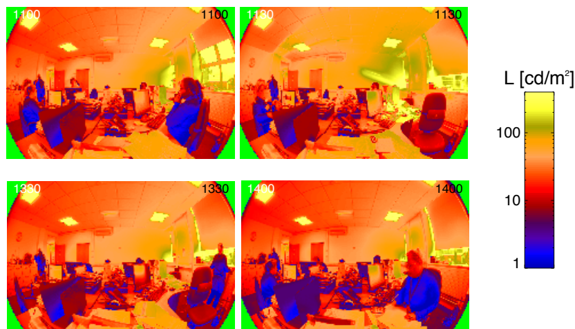
Figure 5. Selected false-colour luminance images from around the time of visual comfort actions (VCAs), morning (top two images) and afternoon (lower two images). Note, the scale of luminance ( \text{cd/m}^2 ) and time stamps are in the corner of each image.
