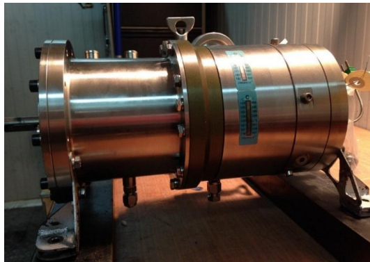
Figure 3. Swash-plate expander delivered by Exoès.
